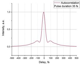
PErL-PM-EHP typical AC envelope at 210 mW, 100 MHz
