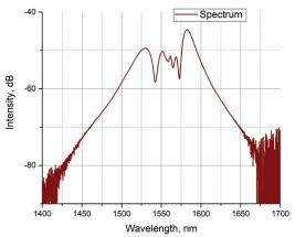
PErL-PM series typical spectrum sample (log scale)
