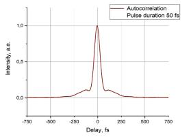
PErL-PM-HP typical AC envelope at 140 mW, 100 MHz
