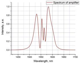
PErL-PM series typical spectrum sample (linear scale)
